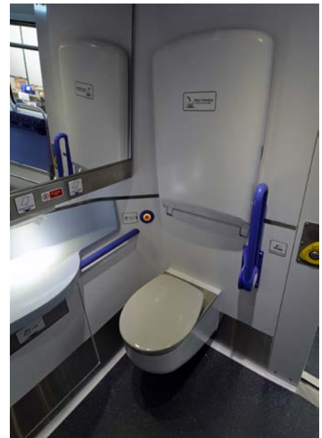
Birley's toilet module is currently being trialled by Porterbrook in their Class 144 Evolution carriage
