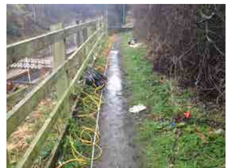
Figure 6-7: Resistivity and seismic surveys being carried out simultaneously (above); results here show the fault zone (5m across with a 5m throw)
