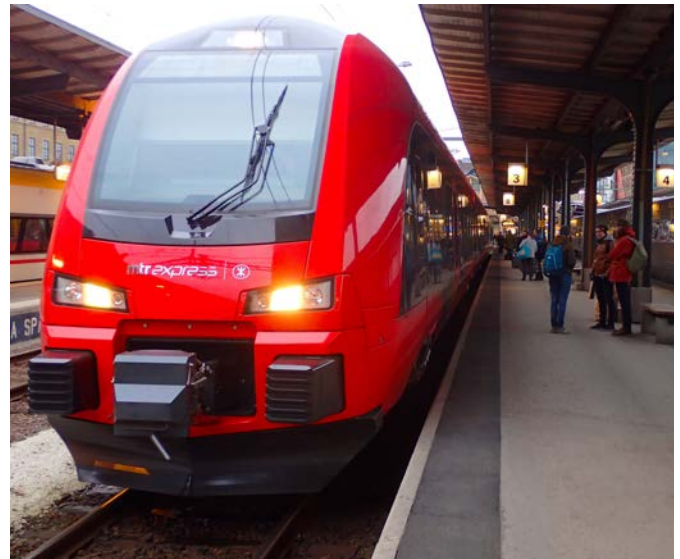
The MTR Express service is run with a total of six brand new FLIRT trains built by Swiss manufacturer Stadler. Each train has five carriages and can carry 244 passengers
