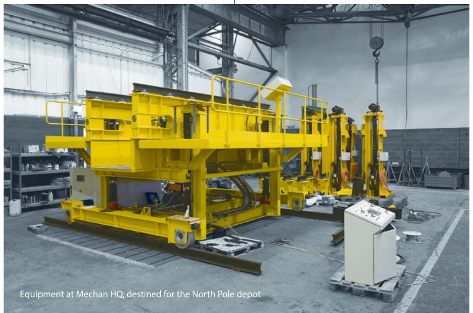
15-tonne jacks at Alstom's depot
