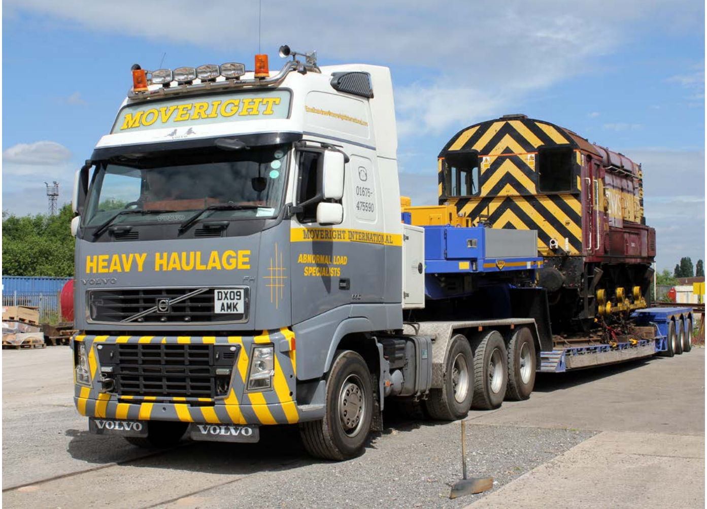
A Moveright International haulage lorry loaded with a Class 08 shunting locomotive
